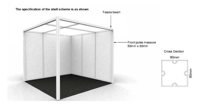
70mm Beam 495mm centres Seen size - 950mm x 2340mm Seen size Cut size - 964mm x 2354mm 455mm x 2340mr Cut size 469mm x 2354mm MODI II AR MODILI AR 80mm x 80mm 455mm between Posts End Post 40mm x40mm Post 70mm Beam 80mm x 80mm
